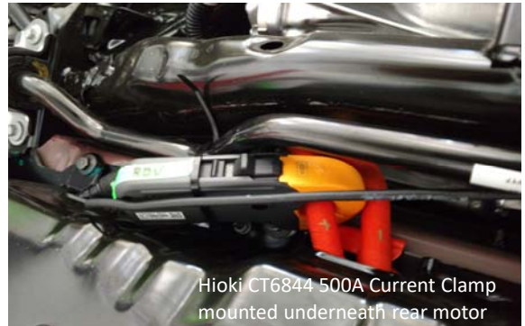
Pic of Hioki connection - High Voltage Ancillaries (Compressor)
