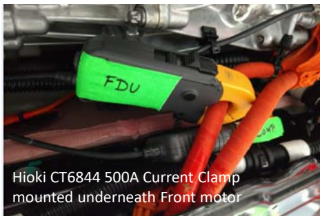
Pic of Hioki connection - DC/ DC to HV BUS
